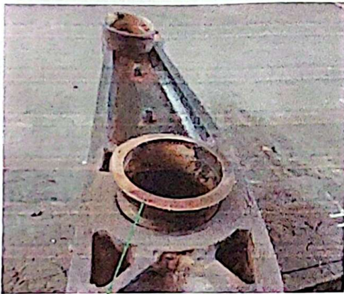
Brush Bush (CPF Item Serial No.03) Size: OD-140 mm, ID-95 mm, Length-230 mm
