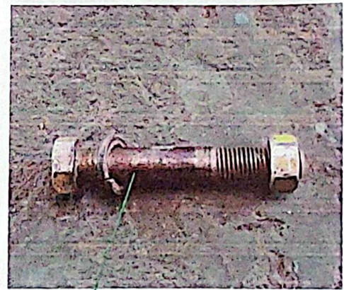
SS Nut Bolt with Spring Washer (CPF Item Serial No.04) Size: Dia-16 mm, Length-120 mm, Thread Length-40 mm
